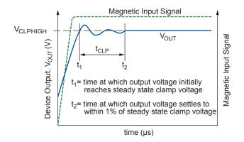
Figure 2. Definition of Delay to Clamp,  $\ensuremath{t_{\text{CLP}}}$
