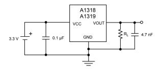
Figure 5. Typical Application Circuit
