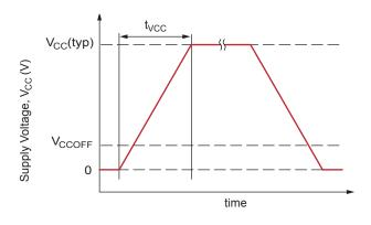
Figure 4. Definition of  $V_{CC}$  Ramp Time,  $t_{VCC}$
