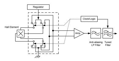
Figure 6. Chopper Stabilization Technique
