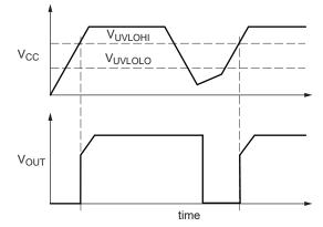
Figure 3. Definition of Undervoltage Lockout
