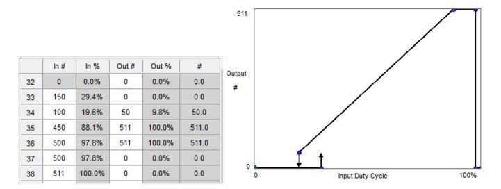
*Example 4:* In this example, the motor won't turn on until the input is about 30% and will turn off when the output falls below about 20%. The output will be at maximum when the input is between about 88% to 98%, and the motor will stop when the input is > 98%.
