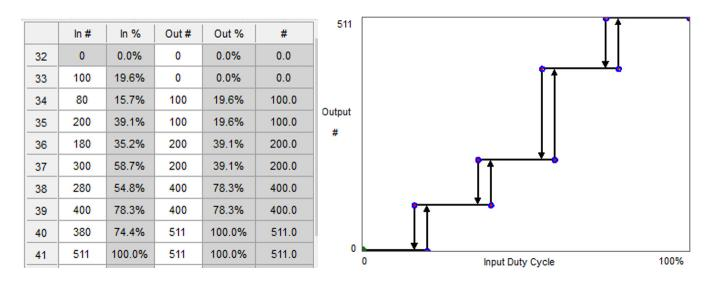
*Example 3:* Hysteresis can be implemented by setting the input value of an address lower than the input value in the previous address. In this example, as the input demand is rising, the output demand will jump to next higher level at the vertical lines on the right of each transition. When the input demand is falling, the output demand will drop to next lower level following the vertical lines on the left of each transition. This prevents output jitter when the input is around a boundary.
