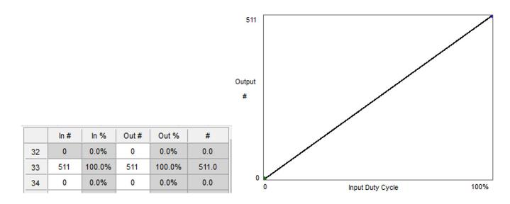
*Example 1:* These screenshots are taken from the A89307 application—white boxes are the entered values. This is the most trivial example, where input = output. This is the curve that is used when the transformer is disabled. Because 511 is the input value in the second address, the 30 following addresses are ignored.
