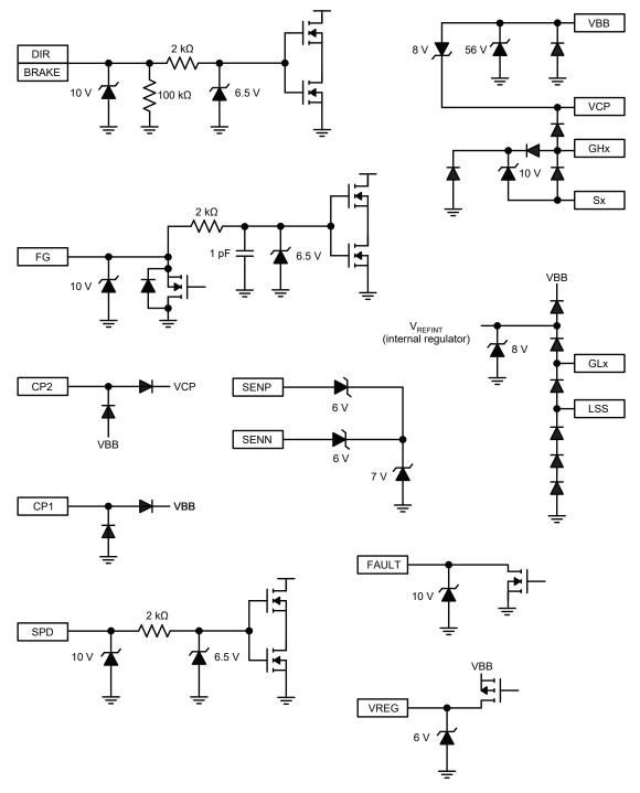
Figure 8: Terminal Diagrams
