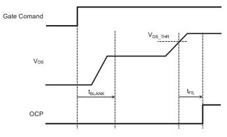
Figure 5: OCP timing diagram
