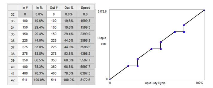
*Example 2:* In this example, the control loop is set to closed-loop speed, and so the resulting rpm is shown in the last column of the table where the curve is defined. This curve is designed to avoid this motor's resonant frequency at 2000 rpm, and its harmonics at 4000 rpm and 6000 rpm.
