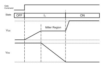
Figure 3: Off-to-On Transition (Slew Rate Control)
