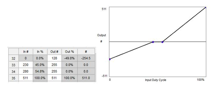
*Example 5:* The curve can be set to control bi-directional operation as well. When the bidirectional option is selected, the output value 511 is still the highest output in one direction, but the output value 255 will stop the motor, and the output value 0 is the highest output in the reverse direction. Here, the motor will run at half speed reverse when input demand is 0, will stop when the input is between 230 and 280, and will run at full speed forward when the input is 511.
