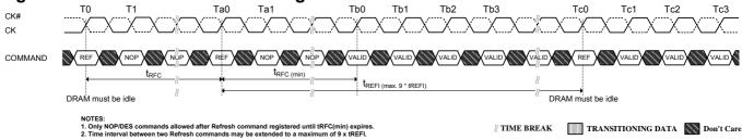
Figure 54. Self-Refresh Entry/Exit Timing
