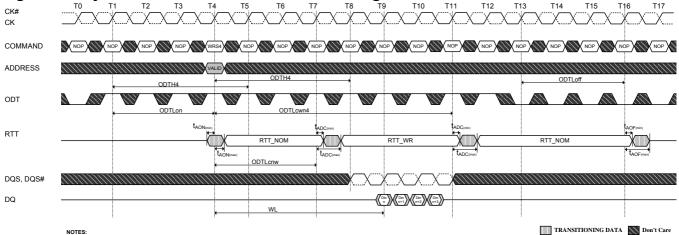
NOTES: Example for BC4 (via MRS or OTF), AL = 0, CWL = 5. ODTH4 applies to first registering ODT high and to the registration of the Write command in this example, ODTH4 would be satisfied if ODT went low at T8 (4 clocks after the Write command).
