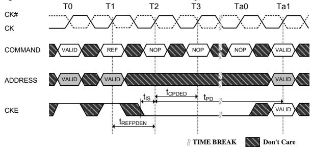
Figure 62. Active Command to Power-Down Entry
