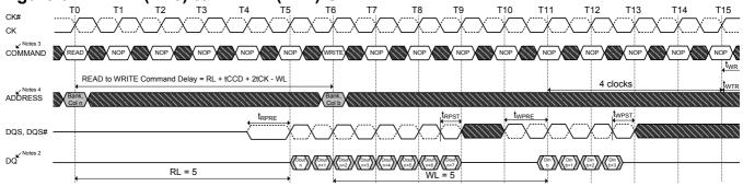
NOTES:  $1. \, RL = 5 \, (CL = 5, \, AL = 0), \, WL = 5 \, (CWL = 5, \, AL = 0) \\ 2. \, DOUT \, n = data-out from column, DIN b = data-in from column b. \\ 3. \, NOP commands are shown for ease of illustration; other commands may be valid at 4. BL8 setting activated by MR0[A1:0 = 01] and A12 = 1 during READ command at T0. BC4 setting activated by MR0[A1:0 = 01] and A12 = 0 during WRITE command at T6.$
