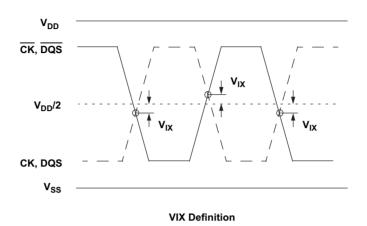
Cross point voltage for differential input signals (CK, DQS): 1.35V
