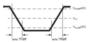
**Differential Output Slew Rate definition**
