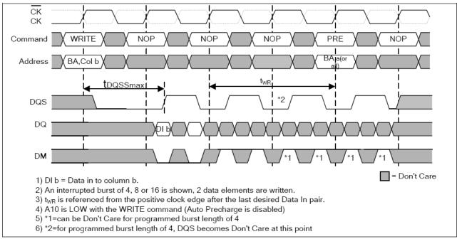
Figure 31 — Interrupting Write to Precharge
