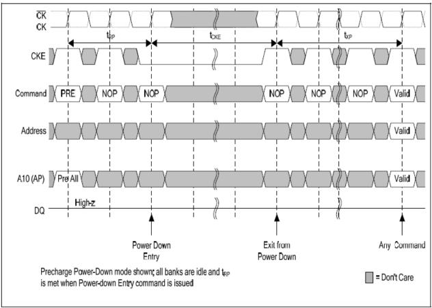
Figure 37 — Power-Down Entry and Exit
