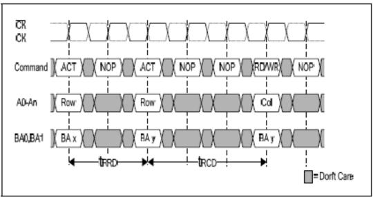
Figure 11 — Bank Activation Command Cycle
