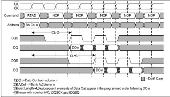
Figure 14 — Read Burst Showing CAS Latency
