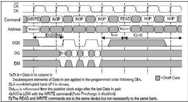
Figure 28 - Non-Interrupting Write to Read
