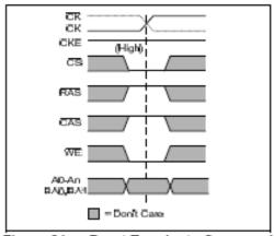
Figure 21 — Burst Terminate Command
