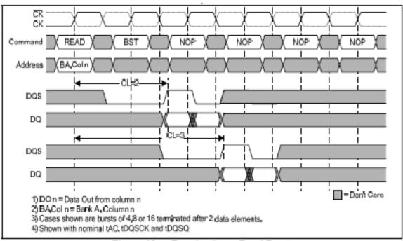
Figure 18 — Terminating a Read Burst
