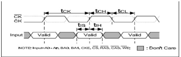
Figure.6 — Basic Timing Parameters
