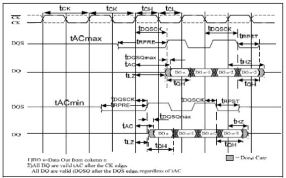
Figure 13 — Basic Read Timing Parameters
