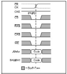
Figure 8 - Mode Register Set Command
