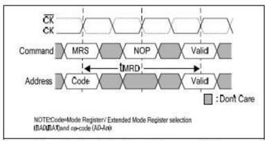
Figure 9 - Mode Register Set Command Timing
