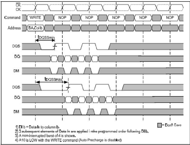
Figure 24 — Write Burst (min. and max. tDQSS)
