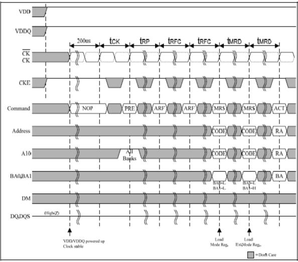
Figure 5 — Initialization Waveform Sequence
