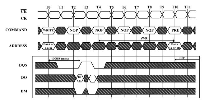
$1\ subsequent\ elements\ of\ Data\ In\ are\ applied\ in\ the\ programmed\ order\ following\ DI\ n$  A non-interrupted burst of  $2\ is\ shown$
