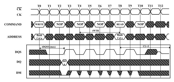
An interrupted burst of 8 is shown, 1 data elements are written
