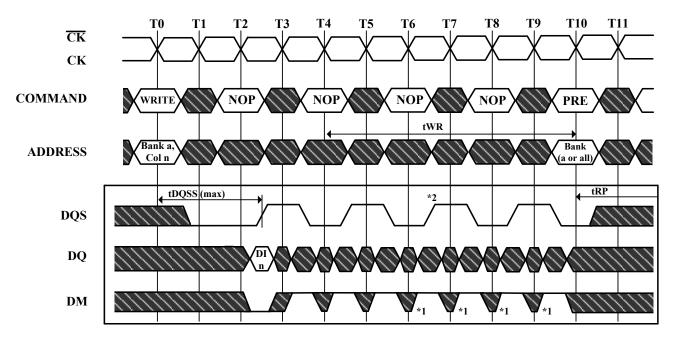
An interrupted burst of 4 or 8 is shown, 1 data element is written tWR is referenced from the first positive CK edge after the last Data In Pair A10 is LOW with the WRITE command (AUTO PRECHARGE is disabled)
