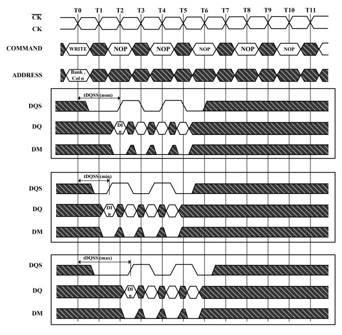
3 subsequent elements of Data are applied in the programmed order following DI n A non-interrupted burst of 4 is shown
