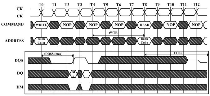
1 subsequent elements of Data In are applied in the programmed order following DI n
