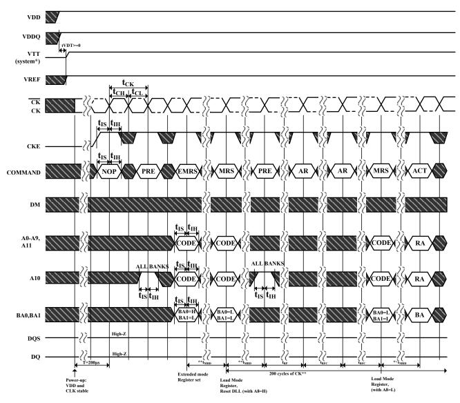
$<sup>^{\</sup>star}\text{=VTT is not applied directly to the device, however tVTD must be greater than or equal to zero to avoid device latch-up}$
