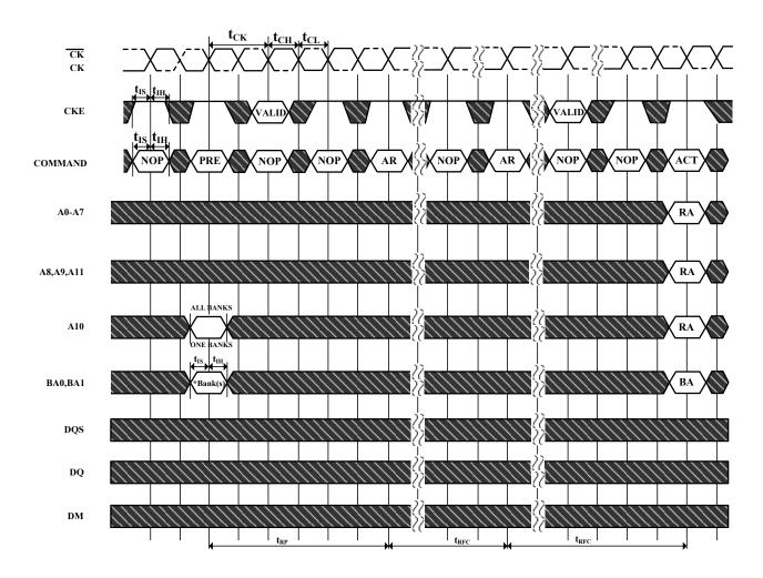
\*= "Don't Care", if A10 is HIGH at this point; A10 must be HIGH if more than one bank is active (i.e., must precharge all active banks)
