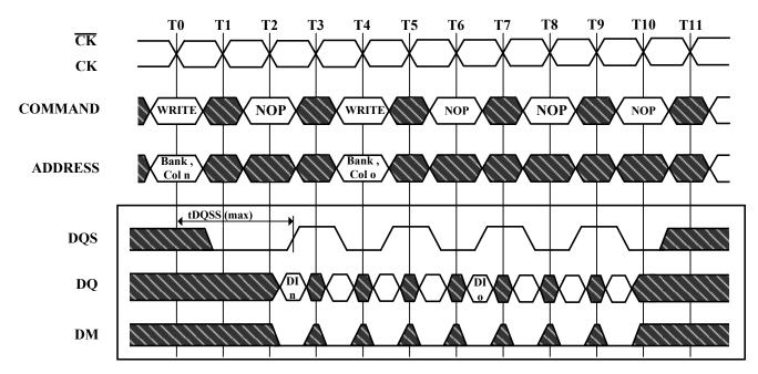
3 subsequent elements of Data In are applied in the programmed order following DI n
