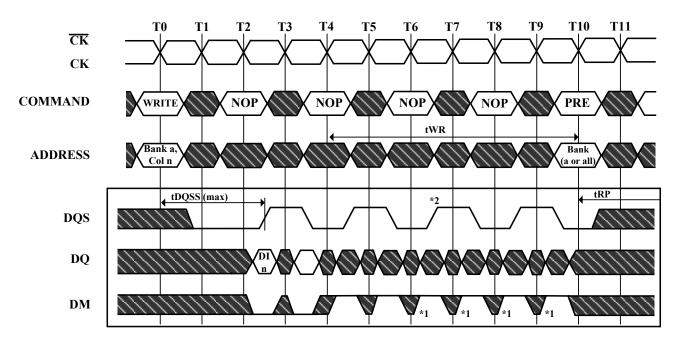
An interrupted burst of 4 or 8 is shown, 2 data elements are written tWR is referenced from the first positive CK edge after the last Data In Pair A10 is LOW with the WRITE command (AUTO PRECHARGE is disabled)
