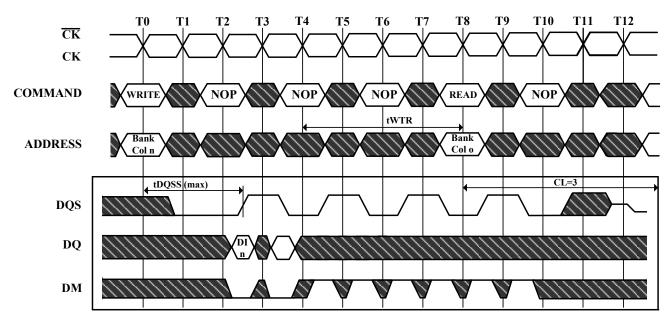
1 subsequent elements of Data In are applied in the programmed order following DI n
