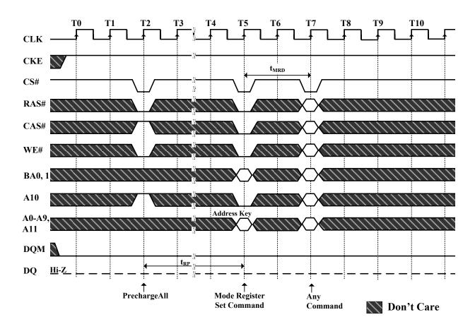
Figure 15. Mode Register Set Cycle
