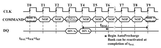
Figure 14. Burst Write with Auto-Precharge (Burst Length = 2)
