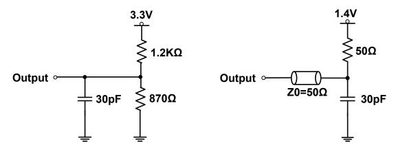
Figure 18.1 LVTTL D.C. Test Load (A)
