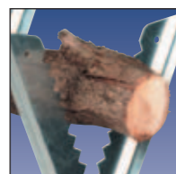
Saw horse: Sturdy support thanks to toothed grippers
