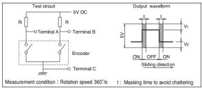
V1=V2=2.5V max. At R =  $5k\Omega$  Chattering: 5ms max. Bounce: 5ms max.
