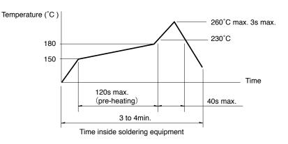
TACT Switch™ / Soldering Conditions
