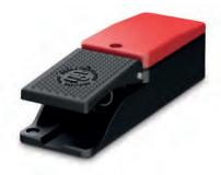
Latching Operation -Push pedal to change contact state. When you release the pedal , the contacts remain in that state. Push again to return to original state. Analog Output Operation -As the pedal is depress, voltage or amperage (depending on model) is increase. Features an additional programmable NP NO signaling contact that activates at a preset level.
