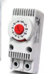
The Heating version (red dial, NC) has closed contacts when the temperature is below the set point value and opens with rising temperature.
