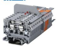
DDFL4U - Double Level Fuse Terminal with fuse link on the top level has a separate feed through terminal at the lower level. This eliminates use of an additional feed through terminal.
