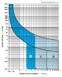
GFL Series RCBO Ground Fault Trip Curve
