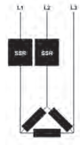
Two-phase SSR SOB to control heaters connected in delta (for high voltage, balanced or unbalanced loads)
