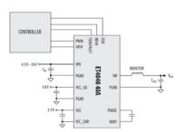
The Enpirion\* ET4040QI is a 40A, high-speed, high-density, monolithic powertrain integrated circuit (IC) with integrated sensing features. It is optimized for low duty cycle operation, making it an ideal solution for FPGA core, processor, or DDR memory applications.
