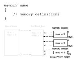
Suppose your embedded system has 512kB of external ROM, named simrom, 512kB of external RAM, named simram and 32kB of external NVRAM, named  $my_nvram$  (see figure above.) All memories are connected to the bus local\_bus. In LSL this looks like follows:
