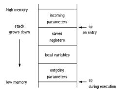
All ARM architectures, except for M-profile architectures, have separate stack pointers for each processor mode. M-profile architectures have one stack pointer. These stack pointers should be initialized at run-time. This is taken care of by the startup code in the run-time library, by means of linker-generated symbols defined in the LSL file. See Section 8.1, *Startup Code*, for a list of these symbols.
