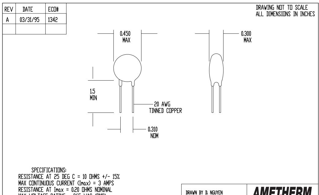
MAX CUNTINUUUS CURRENT (Imax) = 3 AM RESISTANCE AT Imax = 0.20 DHMS NDMINA MAX VOLTAGE RATING = 265 VAC (RMS) MAX SURGE RATING = 17 JOULES ENCAPSULATION = SILICONE RESIN MARKING = DPTIONAL LEADS = RODAN P/N STL-209-14
