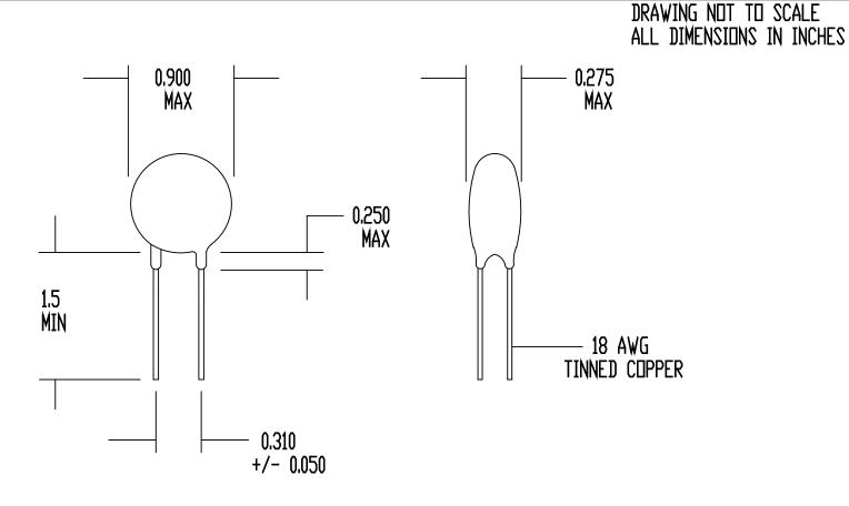
SPECIFICATIONS: RESISTANCE AT 25 DEG C = 5 DHMS +/- 15% MAXIMUM CONTINUOUS CURRENT (Imax) = 12 AMPS RESISTANCE AT Imax = 0.06 DHMS NOMINAL MAXIMUM VOLTAGE RATING = 265 VAC (RMS) MAXIMUM SURGE RATING = 100 JOULES ENCAPSULATION = SILICONE RESIN MARKING = OPTIONAL LEADS = RODAN P/N STL-209-18
