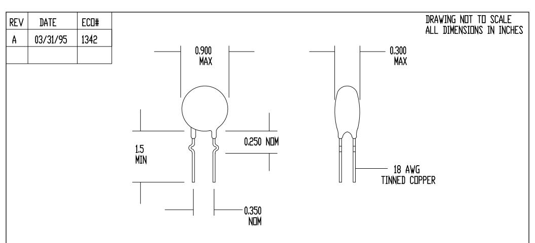
SPECIFICATIONS: RESISTANCE AT 25 DEG C = 2.5 DHMS +/- 15% MAX CONTINUOUS CURRENT (Imax) = 10 AMPS RESISTANCE AT Imax = 0.04 DHMS NOMINAL MAX VOLTAGE RATING = 265 VAC (RMS) MAX SURGE RATING = 87 JOULES ENCAPSULATION = SILICONE RESIN MARKING = DPTIONAL LEADS = RODAN P/N STL-209-45
