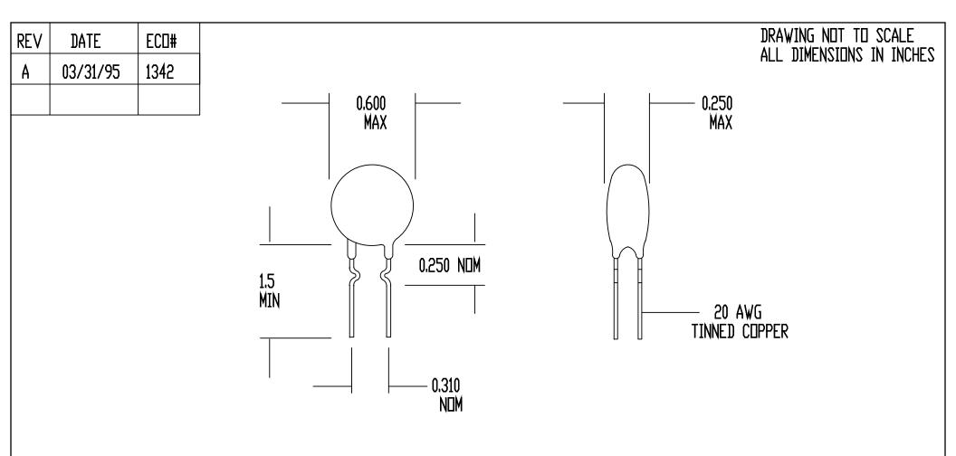
SPECIFICATIONS: RESISTANCE AT 25 DEG C = 5 DHMS +/- 15% MAX CONTINUOUS CURRENT (Imax) = 7 AMPS RESISTANCE AT Imax = 0.07 DHMS NOMINAL MAX VOLTAGE RATING = 265 VAC (RMS) MAX SURGE RATING = 40 JOULES ENCAPSULATION = SILICONE RESIN MARKING = OPTIONAL LEADS = RODAN P/N STL-209-42
