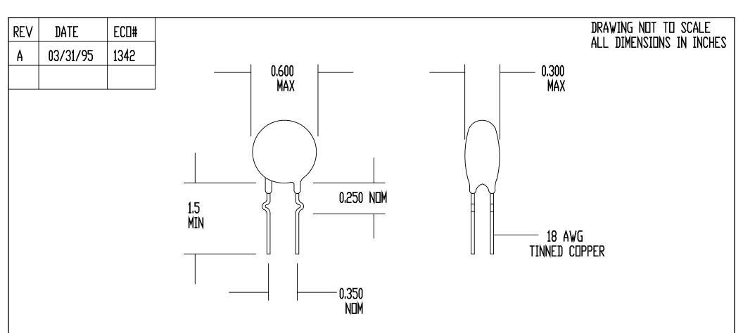
SPECIFICATIONS: RESISTANCE AT 25 DEG C = 7 OHMS +/- 15% MAX CONTINUOUS CURRENT (Imax) = 4 AMPS RESISTANCE AT Imax = 0.20 OHMS NOMINAL MAX VOLTAGE RATING = 265 VAC (RMS) MAX SURGE RATING = 50 JOULES ENCAPSULATION = SILICONE RESIN MARKING = OPTIONAL LEADS = RODAN P/N STL-209-35
