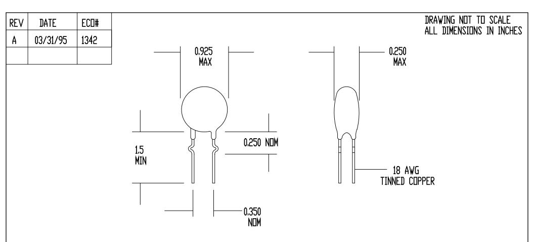
SPECIFICATIONS: RESISTANCE AT 25 DEG C = 120 DHMS +/- 15% MAX CONTINUOUS CURRENT (Imax) = 3 AMPS RESISTANCE AT Imax = 0.90 DHMS NOMINAL MAX VOLTAGE RATING = 265 VAC (RMS) MAX SURGE RATING = 36 JOULES ENCAPSULATION = SILICONE RESIN MARKING = OPTIONAL LEADS = RODAN P/N STL-209-45
