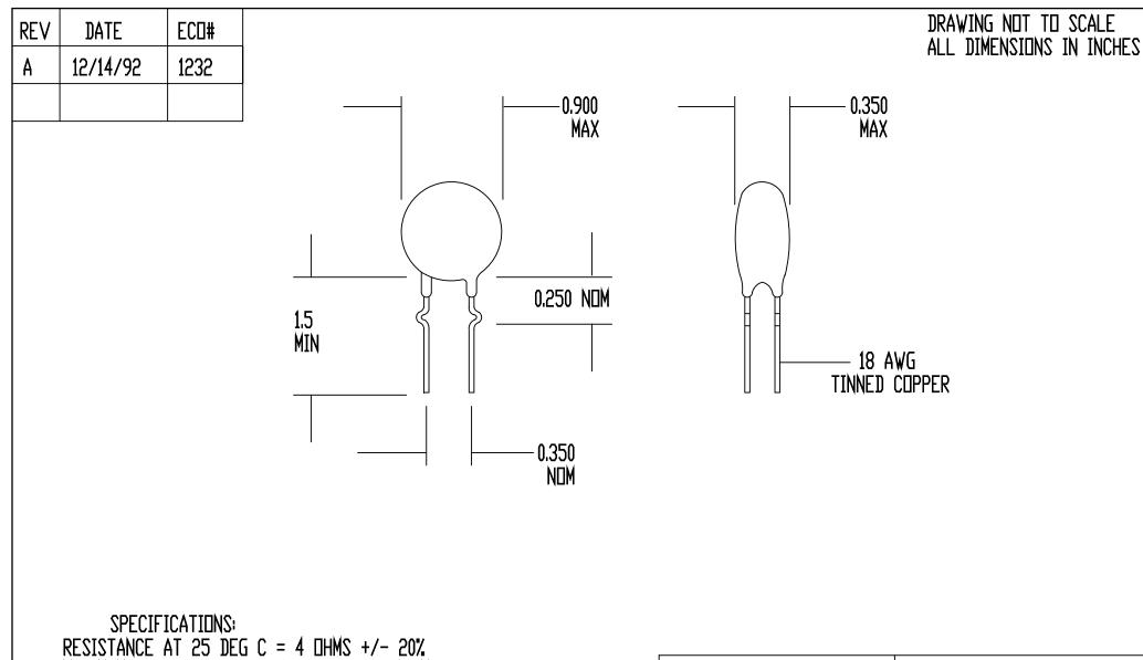
RESISTANCE AT 25 DEG C = 4 DHMS +/- 20% MAXIMUM CONTINUOUS CURRENT (Imax) = 14 AMPS RESISTANCE AT Imax = 0.05 DHMS NOMINAL MAXIMUM VOLTAGE RATING = 265 VAC (RMS) MAXIMUM SURGE RATING = 100 JOULES ENCAPSULATION = SILICONE RESIN MARKING = DPTIONAL LEADS = RODAN P/N STL-209-45
