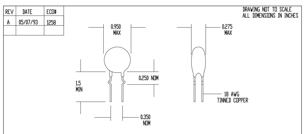
SPECIFICATIONS: RESISTANCE AT 25 DEG C = 7 DHMS +/- 15% MAXIMUM CONTINUOUS CURRENT (Imax) = 10 AMPS RESISTANCE AT Imax = 0.08 DHMS NOMINAL MAXIMUM VOLTAGE RATING = 265 VAC (RMS) MAXIMUM SURGE RATING = 100 JOULES ENCAPSULATION = SILICONE RESIN MARKING = OPTIONAL LEADS = RODAN P/N STL-209-45
