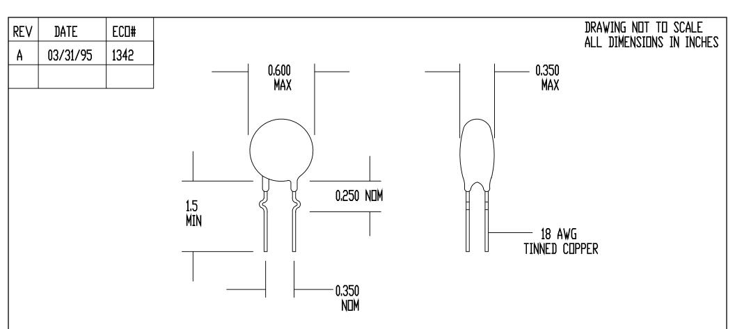
SPECIFICATIONS: RESISTANCE AT 25 DEG C = 10 DHMS +/- 15% MAX CONTINUOUS CURRENT (Imax) = 5 AMPS RESISTANCE AT Imax = 0.20 DHMS NOMINAL MAX VOLTAGE RATING = 265 VAC (RMS) MAX SURGE RATING = 44 JOULES ENCAPSULATION = SILICONE RESIN MARKING = DPTIONAL LEADS = RODAN P/N STL-209-35
