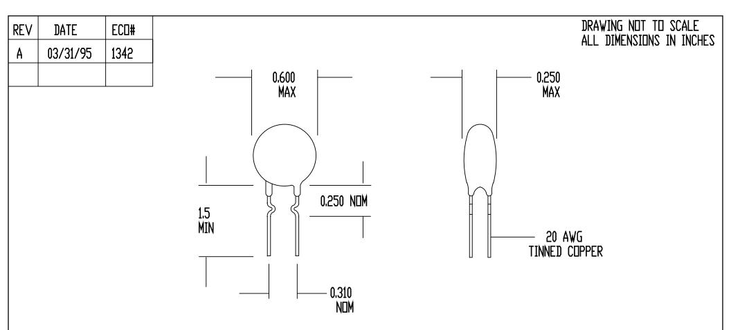
SPECIFICATIONS: RESISTANCE AT 25 DEG C = 60 DHMS +/- 10% MAX CONTINUOUS CURRENT (Imax) = 1.5 AMPS RESISTANCE AT Imax = 1 DHM NOMINAL MAX VOLTAGE RATING = 265 VAC (RMS) MAX SURGE RATING = 50 JOULES ENCAPSULATION = SILICONE RESIN MARKING = OPTIONAL LEADS = RODAN P/N STL-209-42
