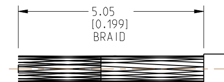
RECOMMENDED CABLE STRIPPING DIMENSIONS (TRIM 1)
