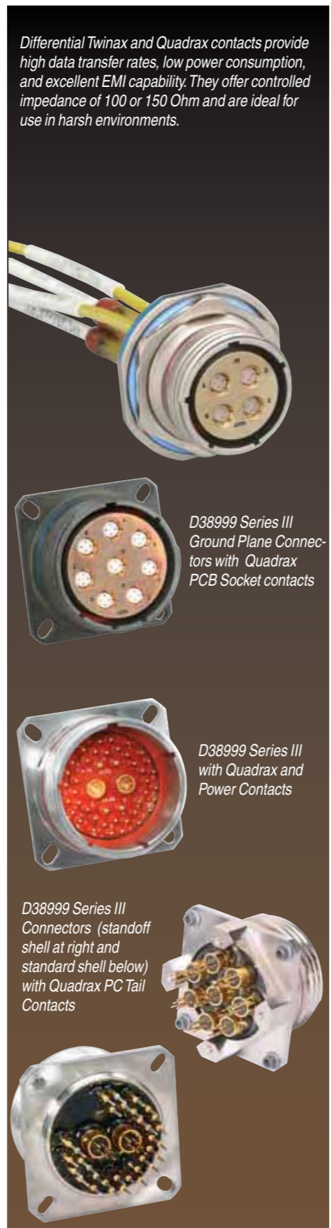
Differential Twinax Contact
