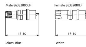
These removable contacts are suitable for the contact cavities of the DMW series and DW series.
