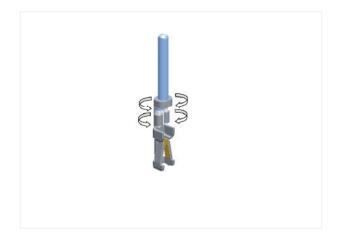
Crimp the terminal onto the wire.
