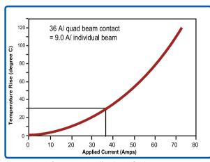
Current rating information is in still air (no air flow) with multiple contacts energized unless otherwise noted
