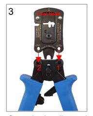
Open the handles and insert the tool head into the open holes.
