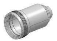
The coupling nut is captivated in the Backshell follower by suitable retention mechanism. This style facilitates the free rotation of the coupling nut and hence assembly of Backshell to the connector becomes easy without turning the entire Backshell body. Lock wire holes are provided on the coupling nut to prevent accidental decoupling when specified.
