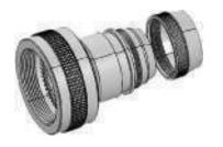
This is another cost effective way to terminate the braid to the adaptor. The braid is pulled over the conical shape to the rear end of the adaptor and tied. The end nut is tightened to ensure adequate grip for the shielding. Heat shrink boot can be used with this adaptor too.
