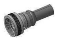
This adaptor is supplied with some length of braid attached. This braid overlaps with the cable braid and effective shielding takes place due to its  $360^{\circ}$  contact. It is designed to accept heat shrink boot. Ease and less time for cable termination are the prime advantages here.
