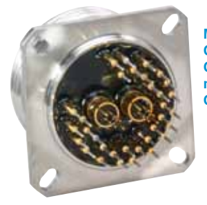
MIL-DTL-38999, SERIES III CONNECTOR WITH PC TAIL CONTACTS. This arrangement has 8 Quadrax PC tail contacts.
