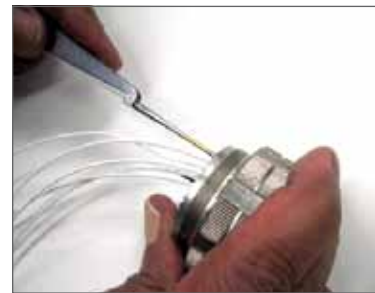
Removal of contacts with metal tool.
