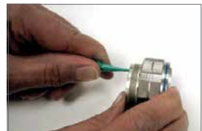
Plastic tool with contact in proper position.
