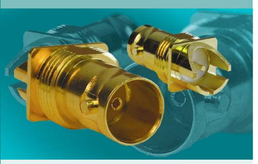
This 75 Ohm BNC bulkhead jack is ideal for use in high-performance video applications. It's end-launch termination saves space in high-density applications where panel real-estate is critical. The industry standard design features gold a gold plated body and PTFE insulator. Nickel plating is also available.
