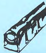
2. Insulation being pierced.
