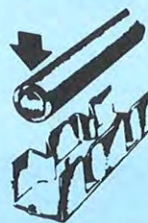
1. Prior to conductor insertion.
