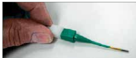
Plastic tool with contact in proper position.
