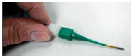
Plastic tool with contact in proper position.
