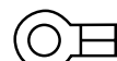
Small Ring for Attaching Receptacle Covers to a Panel with a Screw
