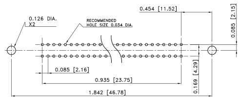
CONTACT HOLE SPACING FOR PC BOARD - RECEPTACLE
