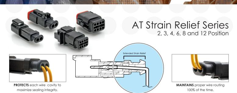
Specifically designed wire cavities protect each individual wire seal, eliminating stress on the rear seal, maintaining IP67 sealing performance regardless of wire bundle direction or improper installation. The AT-SR01 Series is a cost-effective and highly-reliable solution for wire routing, strain relief and sealing issues common in Heavy Duty applications. It ensures a complete environmental seal and necessary strain relief on the production line and in the field.
