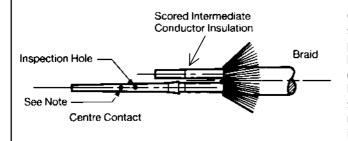
Crimp centre contact (Pin or Socket) on to the stripped wire using tool M22520/2-01 and crimp positioner 294GB-5027-1 (setting No. 4 for 24AWG) butting rear end of contact to wire insulation. The conductor end should be visible in the inspection hole. Note: A second hole is permissible in the socket contact for manufacturing purposes. It is not required to be on the same centre line as the inspection hole.
