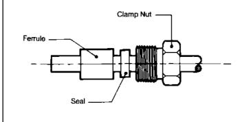
Slide clamp nut, seal and ferrule over cable. (Nut & seal only applicable on single way connector).
