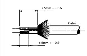
Remove outer sheath of cable to 7.5mm comb out all braids evenly and fold back. Remove cable fillers from stripped length. Strip the centre contact conductor to 4.5mm. Note: It is recommended that both intermediate and centre contact conductors are scored at the correct stripping length. The intermediate conductor insulation should not be removed until the centre contact has been crimped.
