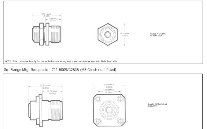
NOTE: This connector is only for use with discrete wiring and is not suitable for use with Data Bus cable.
