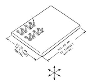
NOTE: Printed Wiring Board to be rigidly mounted along four edges.
