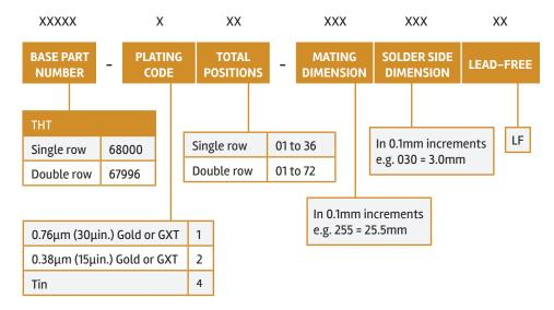
Note: 1. The total combined dimension for mating and solder side may not exceed 27mm
