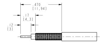
RECOMMENDED CABLE STRIPPING DIM'S. SCALE 3.000
