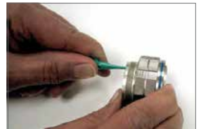
Plastic tool with contact in proper position.
