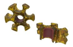
Power Feeder Spacers separate and provide a constant spacing between the power feeders. The custom design of this product allows a six degree rotation on the power feeder bundle and doesn't fight against the natural flow of the cable. It is designed to sit within Omega Clamps which can be used as anchor points.
